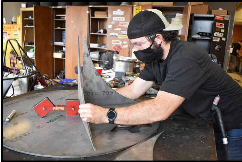
Figure 13 Gusset Alignment Pre-Welding
