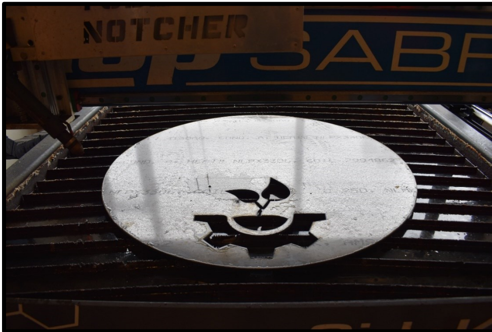
Figure 10 Structure’s Base Following Plasma Cutter Service
